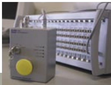
DSCU-DAC Shutdown Control Unit: Safety device, offering manual test abort function with connectivity to external safety devices. The use of a removable hardware key prevents unauthorized usage.
